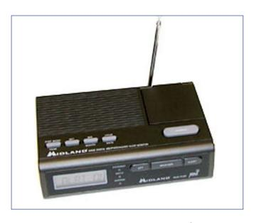
codes are added to each broadcast to identify the event (tornado, flash flood, local civil emergency, etc.) and the specific counties affected. When the warning is received, the receiver turns itself on, sounds an alarm, activates a warning light, writes a short message (TORNADO) on the display, and activates connected external devices, strobe lights, sirens, vibrators, etc.
